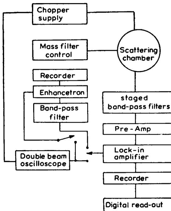
**Figure 1.** Block diagram of the electronics. For the Aberth gun, the mass spectrometer control is replaced by Kepco and Fluke voltage supplies. The enhancetron is connected to the HR-8 Signal monitor.
