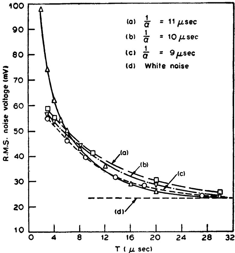
Figure 5. Plot of output noise voltage vs time between triggers ( $T$ ) for exponentially correlated noise with  $\alpha = (\text{RC})^{-1}$ . The solid curve represents the measured data while the dashed curves are based on calculations
