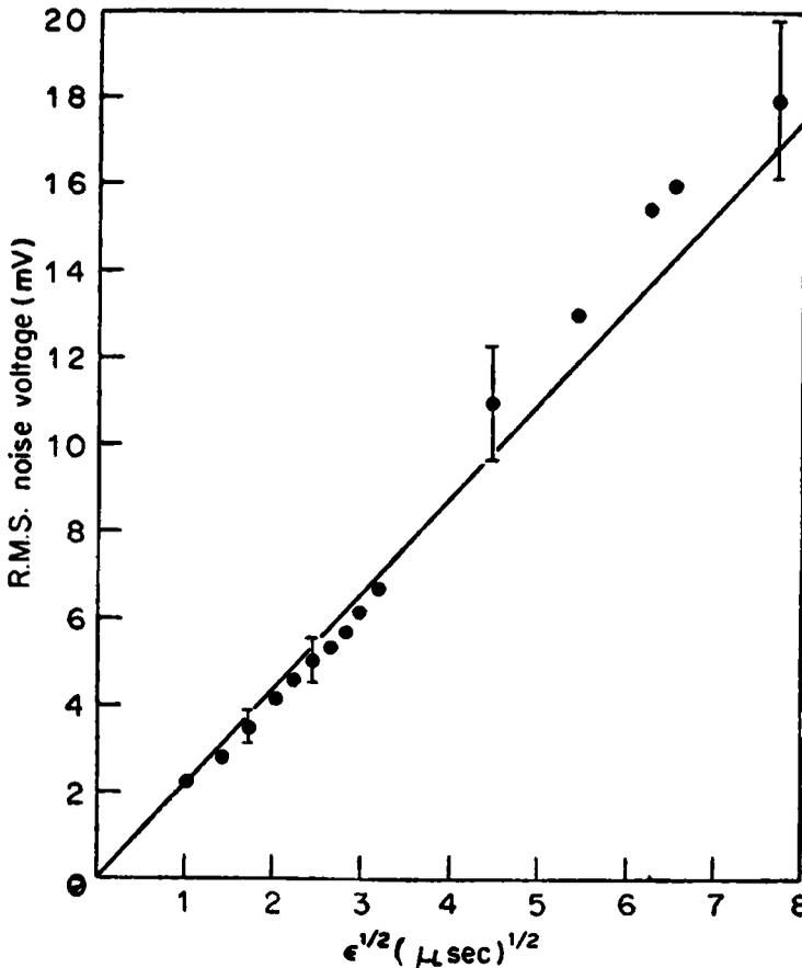
Figure 4. Plot of measured output noise voltage vs  $\epsilon^{1/2}$  for a white noise source
