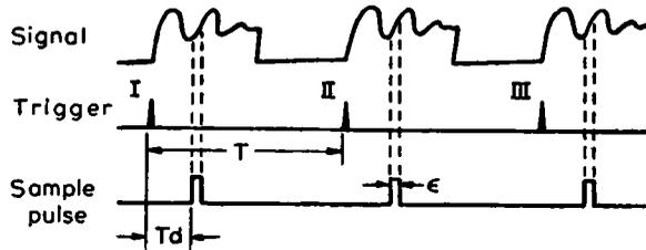
**Figure 2.** Timing diagram of Box-Car averager
