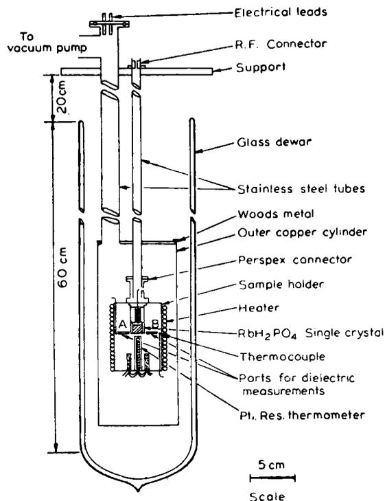
Figure 1. The cryostat.
