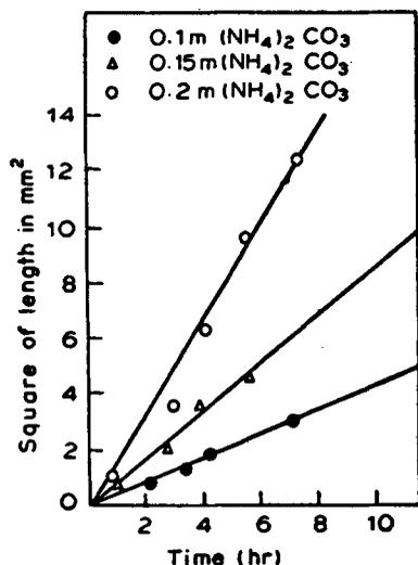
Figure 5. Plot of square of the length of whiskers vs time of growth for whiskers at different  $(\text{NH}_4)_2\text{CO}_3$  concentrations.
