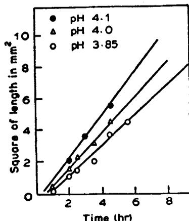
Figure 6. Plot of square of the length of whiskers vs time of growth for whiskers grown in gels of various pH values.
