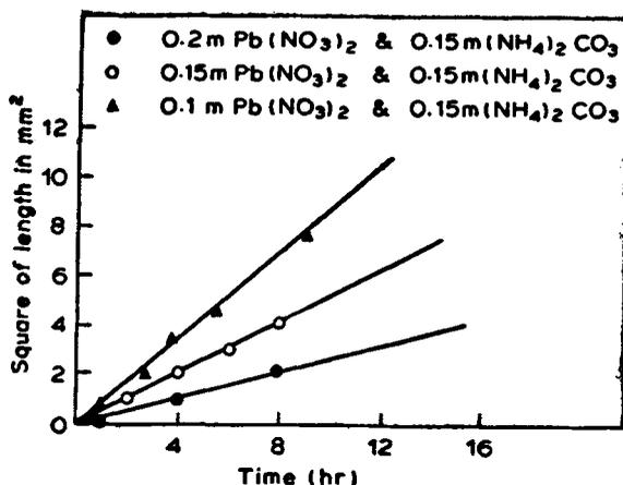
Figure 4. Plot of square of the length of whiskers vs time of growth for whiskers grown in gels of different lead nitrate concentrations.
