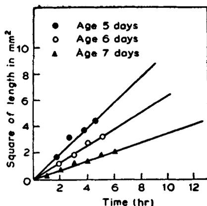
Figure 3. Plot of square of the length of whiskers vs time of growth for whiskers grown in gels of different ages
