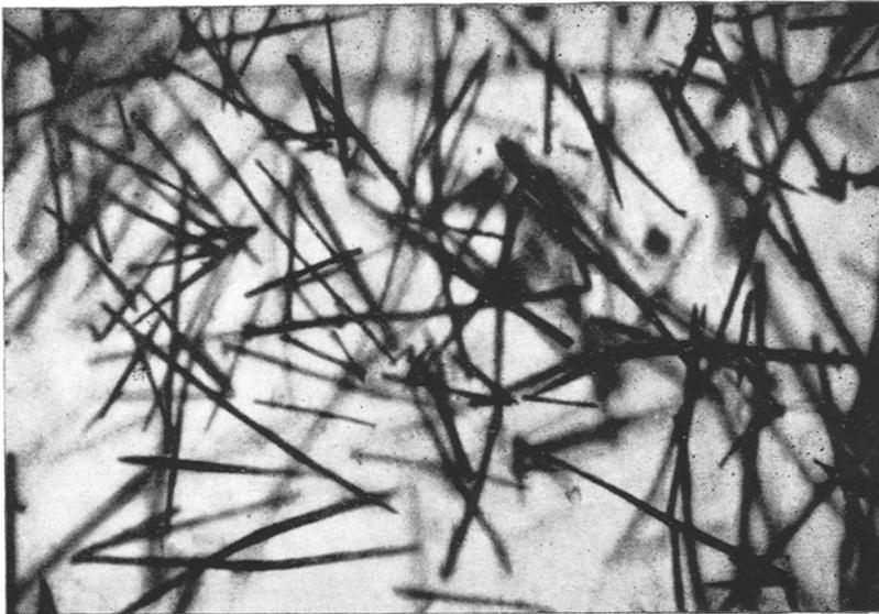
**Figure 1.** Lead carbonate whiskers ( $\times 25$ )
