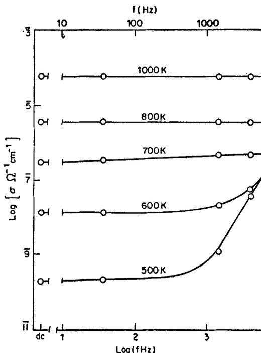
Figure 2. Plot of Logarithm of electrical conductivity ( $\sigma$   $\text{ohm}^{-1} \text{cm}^{-1}$ ) vs log of frequency for pressed pellet of  $Nd_2O_3$  at different temperature.
