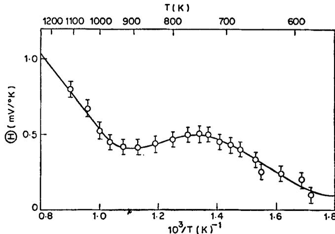
Figure 1. Plot of thermoelectric power ( $\Theta$  mV/K) vs inverse of temperature ( $1/T$ (K)<sup>-1</sup>) for pressed pellet of Nd<sub>2</sub>O<sub>3</sub>.
