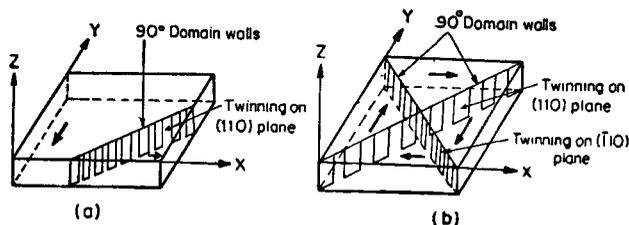
Figure 1. (a) Twinning and (b) Possible twinning on (110) and  $(\bar{1}10)$  planes of the true cell or subcell and the associated domain structure.
