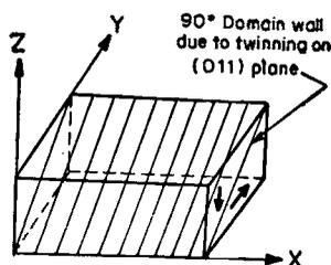
Figure 2. Disallowed  $90^\circ$  domain walls due to twinning on (011) planes
