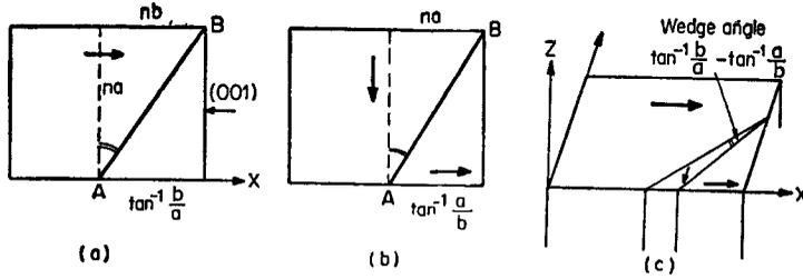
Figure 6. Domain line AB inclined with X axis at (a)  $90^\circ - \tan^{-1}(b/a)$  (b)  $90 - \tan^{-1}(a/b)$  (c) Wedge-shaped domain with wedge angle  $\tan^{-1}(b/a) - \tan^{-1}(a/b)$ .
