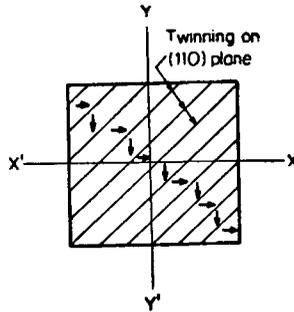
Figure 9. Domain structure present in the crystal shown in figure 8.
