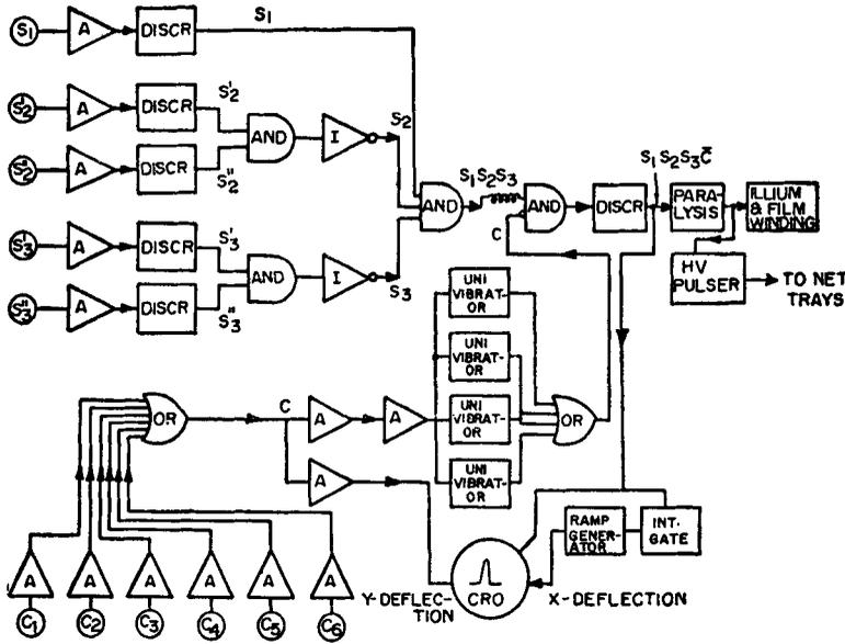
Figure 2. A block diagram of the electronics employed in the experiment to detect heavy leptons.
