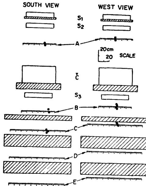
Figure 5. A sketch of an event of the type CD recorded in this experiment. The sub-relativistic particle is well within the geometry penetrating  $S_1$ ,  $S_2$ ,  $\check{C}$ ,  $S_3$  and the first three iron absorbers. It stops in the absorber between the pair of NFTs C and D.
