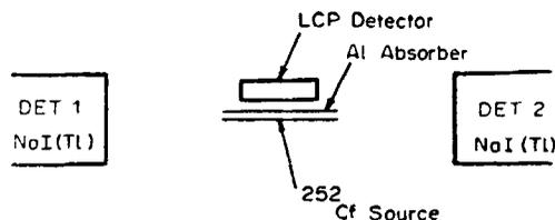
Figure 1. Schematic diagram of the experimental assembly.
