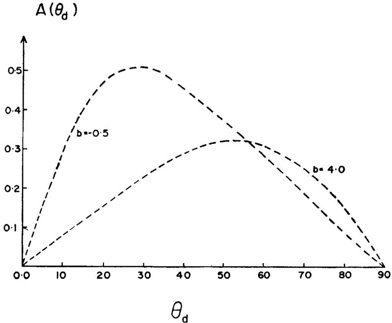
Figure 1. The asymmetry function  $A(\theta)$  as a function of the laboratory angle of the recoil deuteron in  $\nu d \rightarrow \nu d$ , for  $b = -0.5$  and  $b = 4.0$ .
