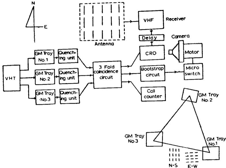
Figure 1. Flow-diagram of the EAS experiment.
