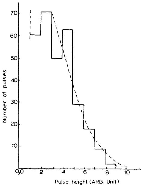
Figure 3. Pulse height distribution of radio pulses at 30 MHz.
