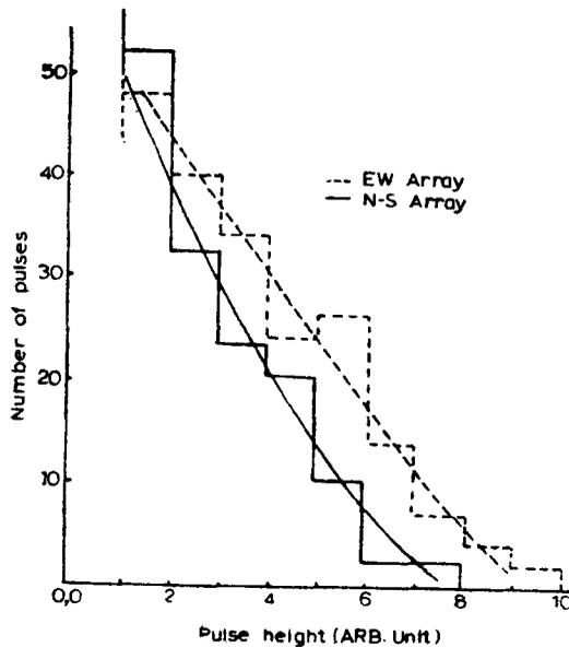
**Figure 5.** Pulse height distribution of radio pulses at 60 MHz (N-S and E-W array).
