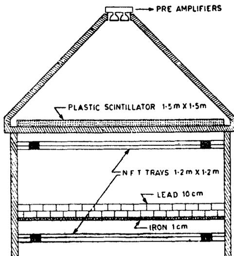
Figure 1. Schematics of the penetrating particle detector, located underground at depth of 580 m.w.e.
