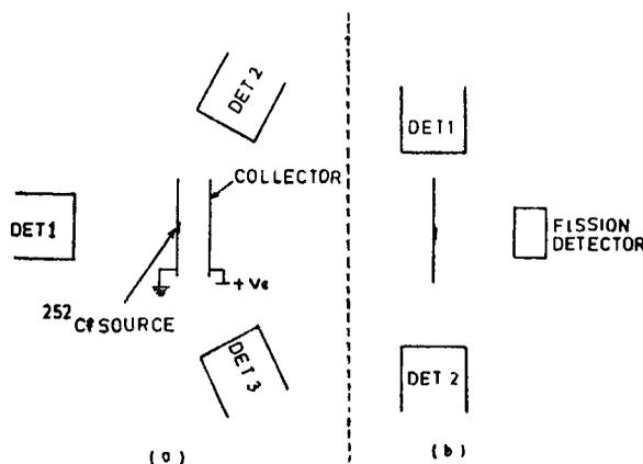
Figure 1. Schematic diagram of the experimental assembly.
