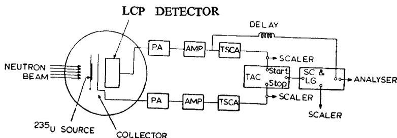
Figure 1. Block diagram of the electronic set-up.
