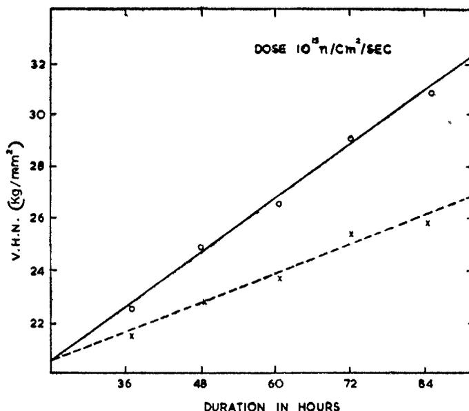
Figure 4. Graph showing hardness measurements of irradiated crystals of all dosages before (solid line) and after heat treatment (dashed line).
