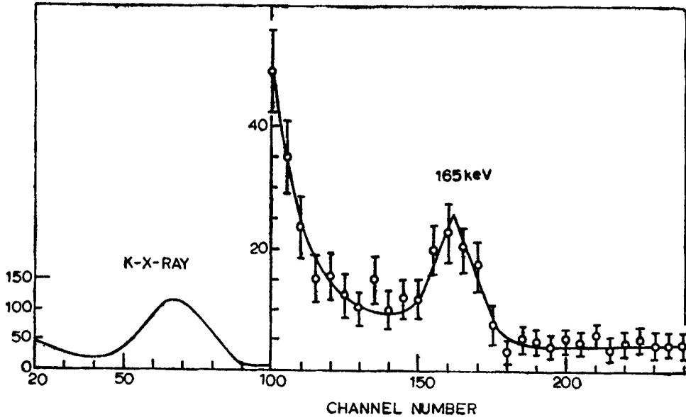
Figure 3. Coincidence spectrum in the Ge(Li) detector with 134 keV selected in NaI(Tl) gate.
