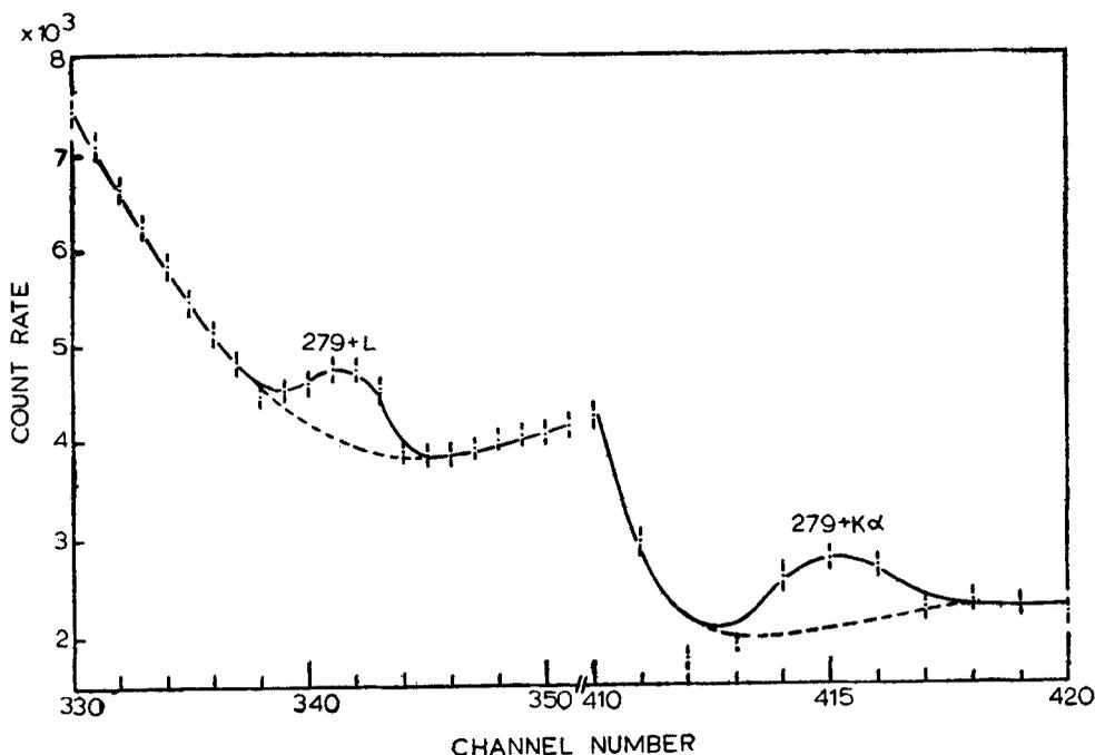
Figure 4. Part of the Ge(Li) spectrum showing  $279 + L$  and  $279 + K_{\alpha}$  lines recorded in close geometry.
