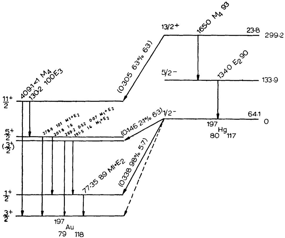
Figure 1. Decay scheme of the radioactive isotope  $^{197m}\text{Hg}$ .
