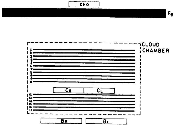
Figure 1. A schematic diagram of the cloud chamber-timing detector system.
