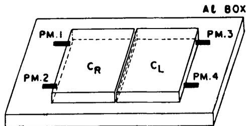
Figure 2. A schematic diagram of the hadron detectors used inside the cloud chamber.
