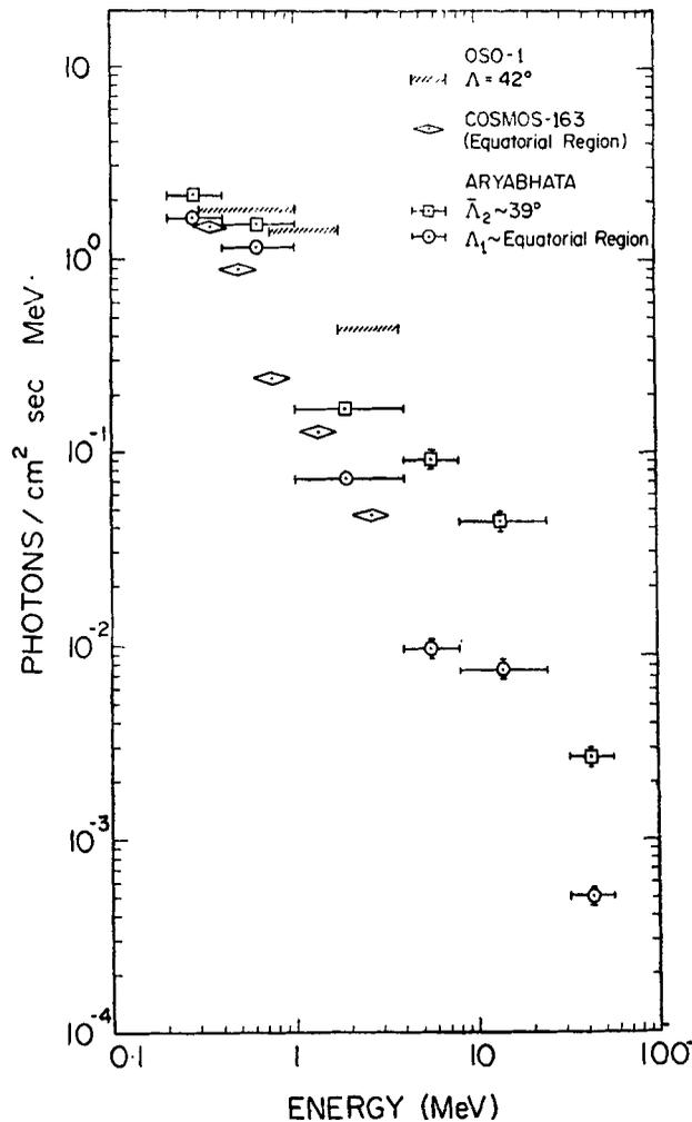
**Figure 3.** The photon spectrum for the gamma ray background, over high latitude ( $\bar{\Lambda} \approx 39^\circ$ ,  $\bar{R}_0 \approx 5.6$  GV), and over equatorial latitudes ( $\bar{\Lambda} \approx 0^\circ$ ,  $\bar{R}_0 \approx 17$  GV) observed in the present experiment on Aryabhata Satellite ( $\sim 600$  km altitude). The data from OSO-1 ( $\sim 550$  km altitude) and COSMOS-163 (apogee: 660 km., perigee: 250 km) satellites are also shown.
