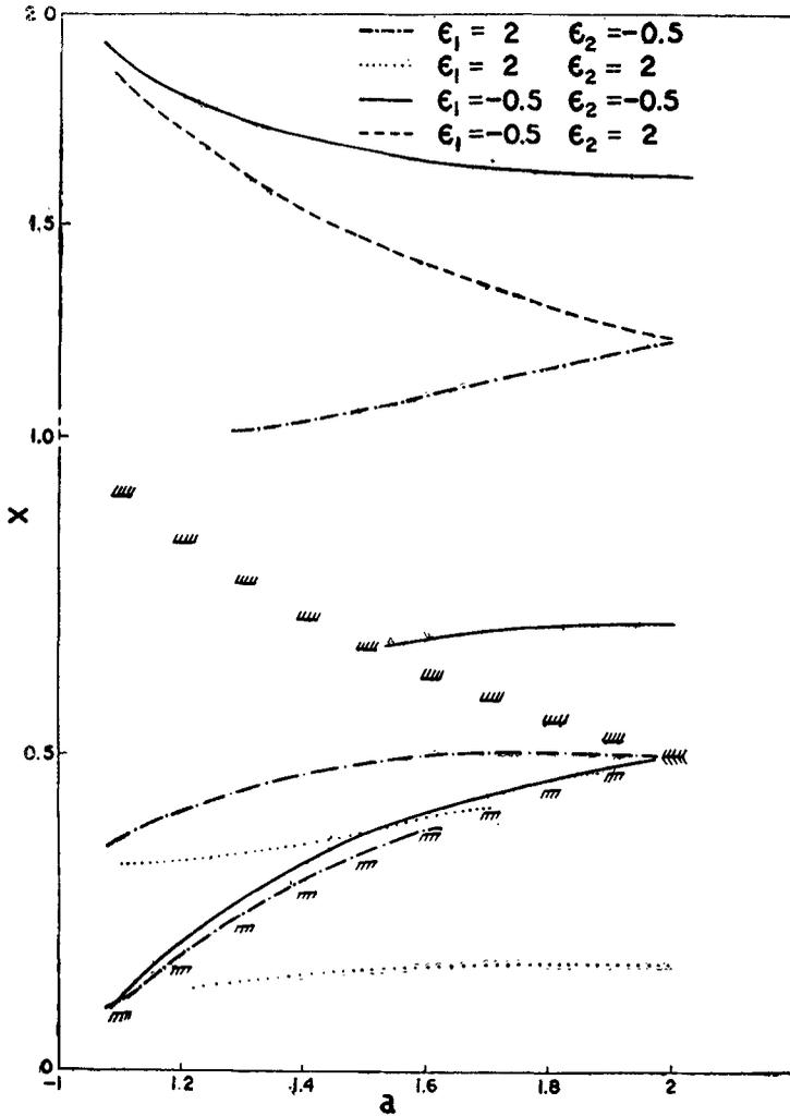
Figure 4. Variation of the impurity pair mode frequencies with the gap in the host crystal is shown. (Note change of scale below and above  $x = 1$ ).
