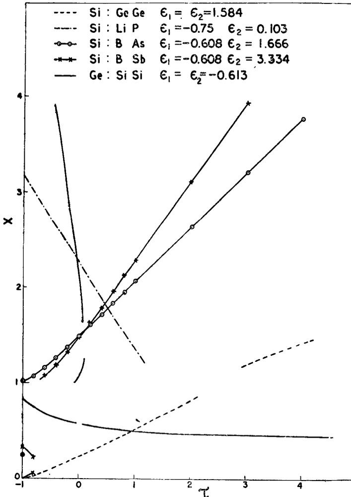
Figure 3. Variation of the impurity pair mode frequencies as a function of  $\tau$  for impurities substituted in Si and Ge hosts.
