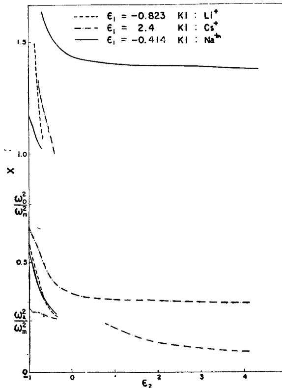
**Figure 1.** Variation of the impurity pair mode frequencies as a function of  $\epsilon_2$  for the mass defect case ( $\tau = 0$ ).
