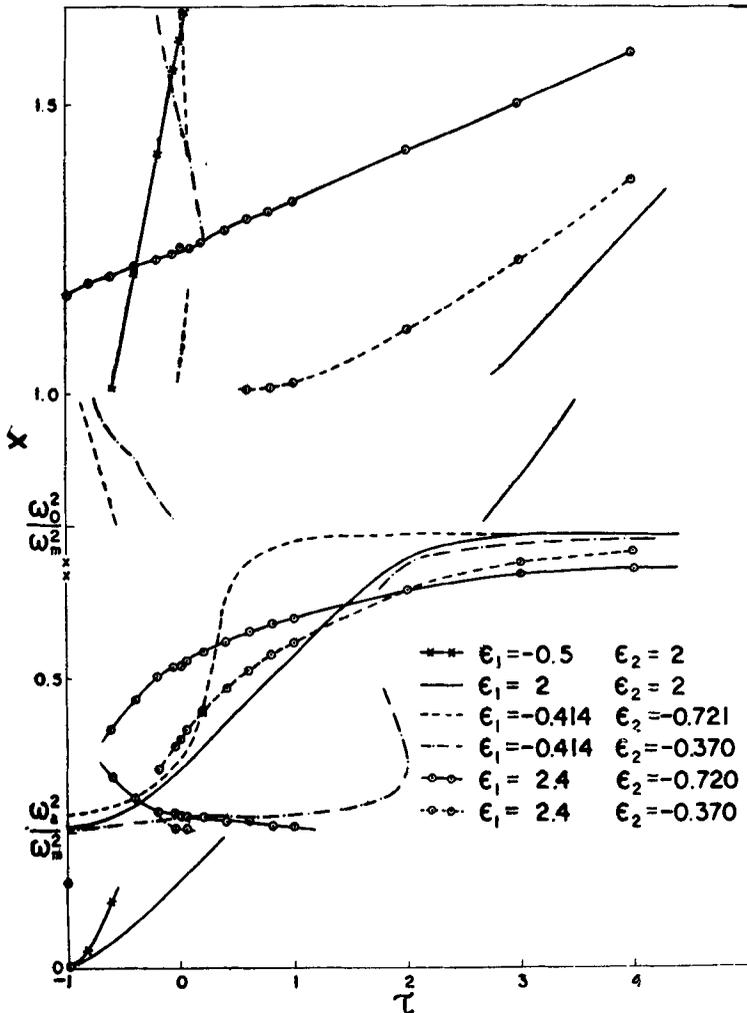
Figure 2. Variation of the impurity pair mode frequencies as a function of the force-constant change parameter  $\tau$ , for a given pair of mass defect impurities substituted in KI.
