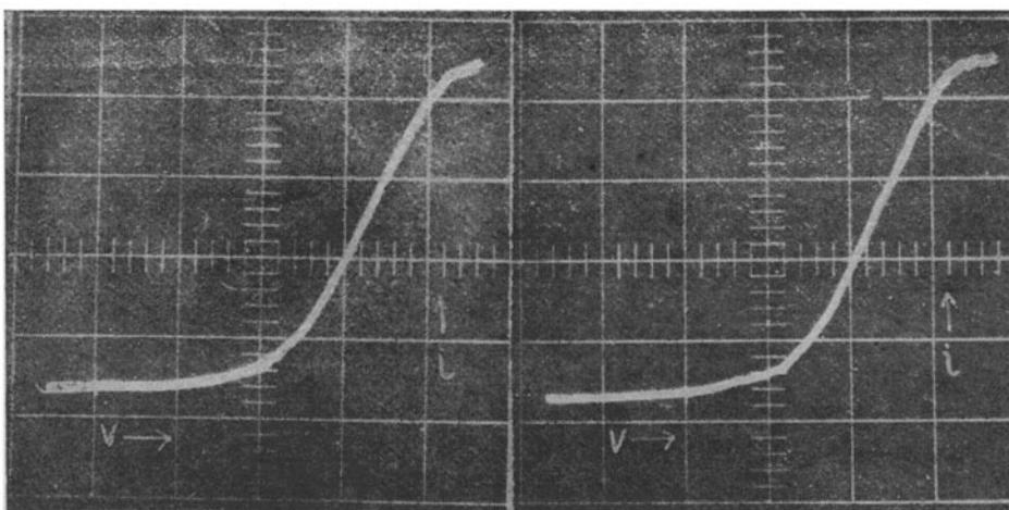
Figure 2. Examples of 'V - i' characteristics as recorded on the CRO screen.
