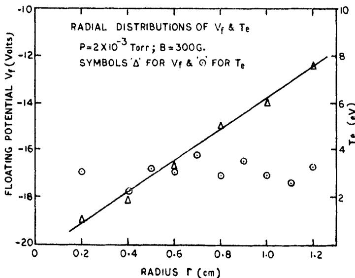
Figure 3.  $T_e$  and  $V_f$  distributions at pressure  $2 \times 10^{-3}$  Torr and magnetic field 300 G.
