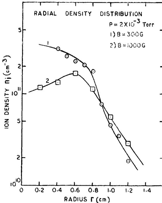
Figure 4. Two examples of ion density,  $n_i$ , distributions at pressure  $2 \times 10^{-3}$  Torr and magnetic fields 300 G and 1000 G.
