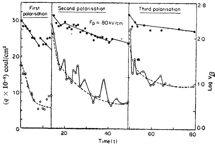
Figure 3. Charge decay of a radio-electret which was repolarized by repeated irradiation.
