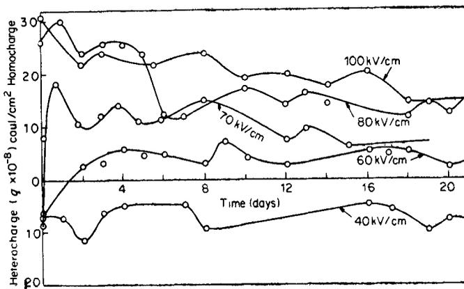
Figure 2. Charge decay of radio-electrets of fluorocarbon.
