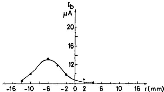
Figure 13. Beam density distribution of the ion source beam (without acceleration).
