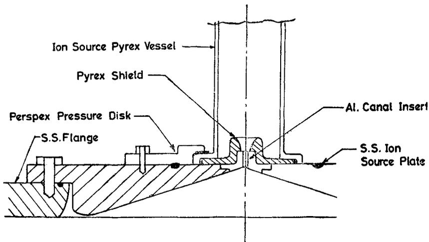
Figure 6. Extraction electrode of the ion source.
