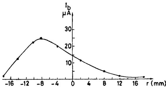
Figure 11. Beam density distribution of the accelerated beam ( $V_{acc} = 30$  kv).
