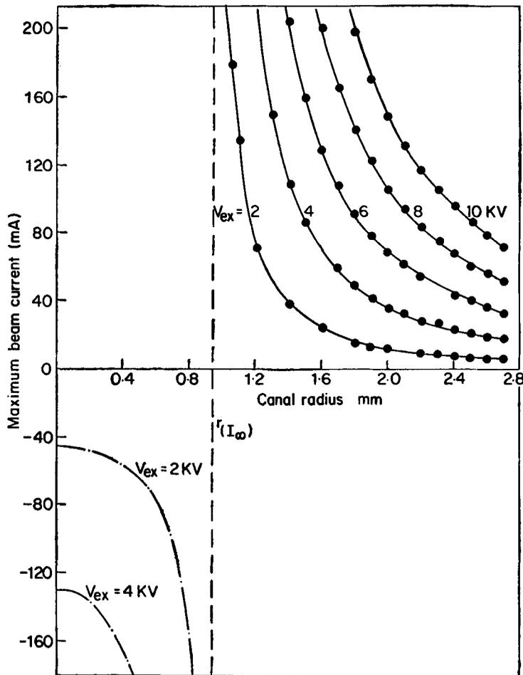
Figure 3. Canal design chart for constant gas consumption ( $G = 30$  cc/hr,  $P = 5 \mu$ ).
