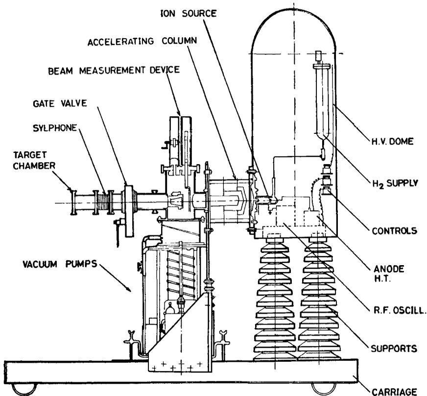
Figure 1. Schematic arrangement of the 150-keV accelerator.
