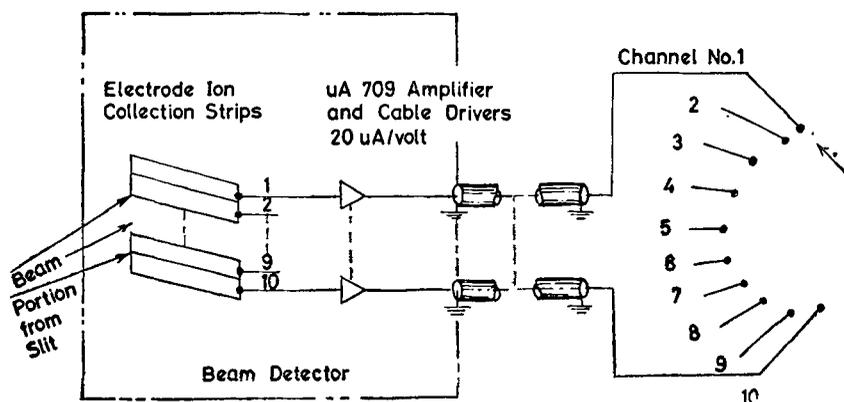
Figure 7 a. Strip electrode arrangement for beam analysis and emittance.
