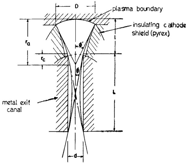
Figure 2. Beam profile in the extraction electrode.
