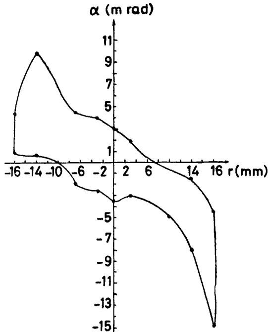
Figure 12. Beam emittance diagram of the accelerated beam (corresponding to figure 11).
