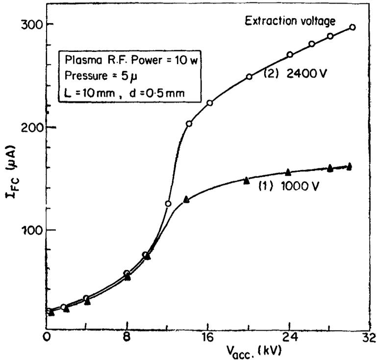
Figure 10. Variation of collected beam current with acceleration voltage.
