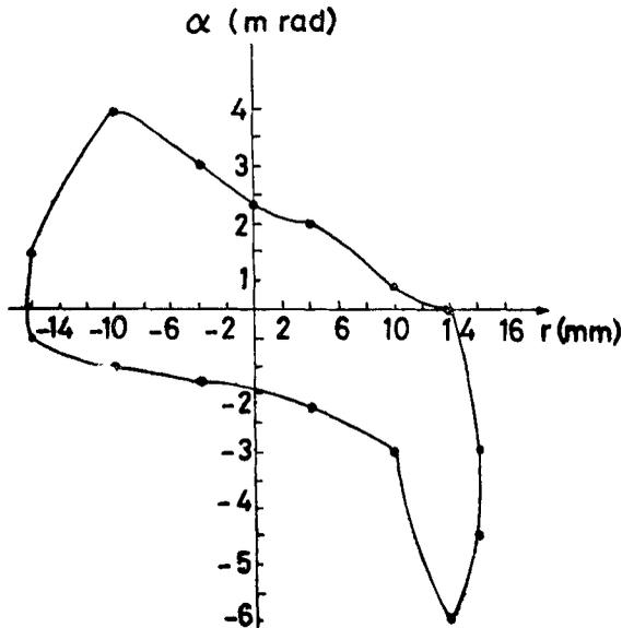
Figure 14. Beam emittance diagram of the ion source beam of figure 13.
