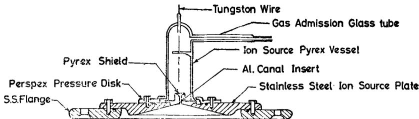
Figure 5. Ion source assembly.
