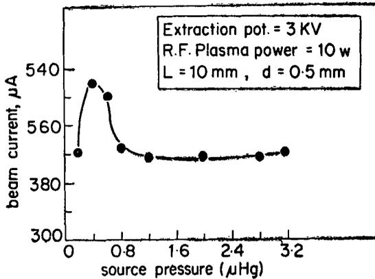
Figure 9. Variation of beam current with gas pressure in the source.
