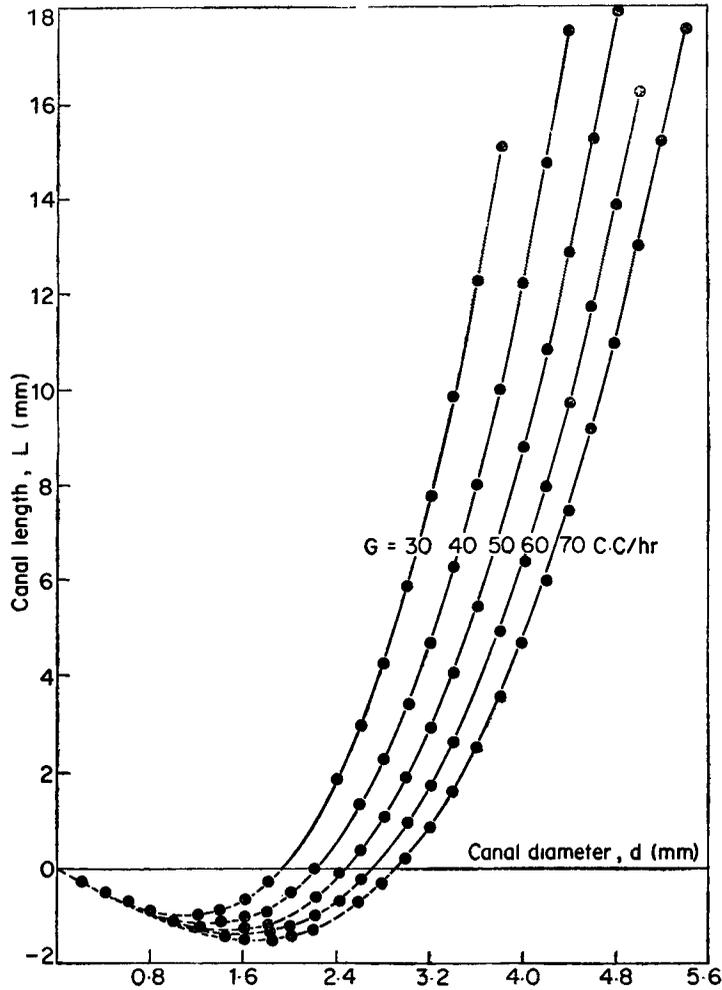
Figure 4. Variation of canal length with its diameter for constant gas consumption.
