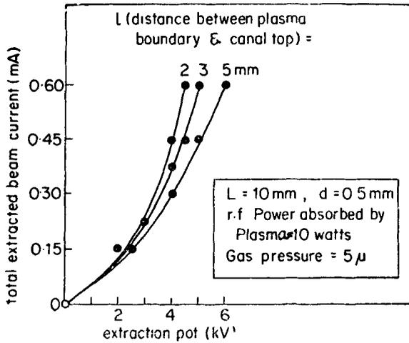
Figure 8. Variation of ion beam current with extraction voltage for different values of spacing above canal top.
