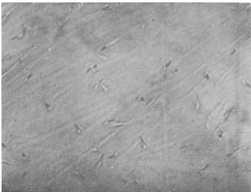
**Figure 1.** Fission tracks in hornblende (Etched for 25 sec at 60° C in 48% HF)
