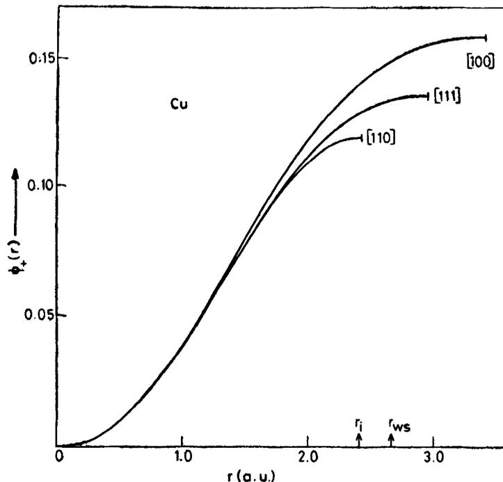
Figure 1. Positron wavefunction along three directions in copper.
