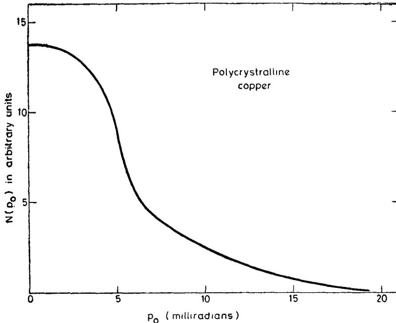
Figure 3. Calculated point slit angular correlation curves for polycrystalline copper.
