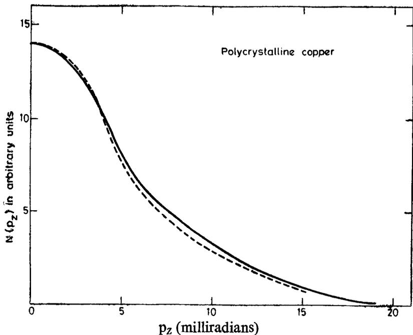
Figure 2. Comparison between the calculated and experimental long slit angular correlation curves for polycrystalline copper. — — — Berko *et al* (1968) and — Theory.
