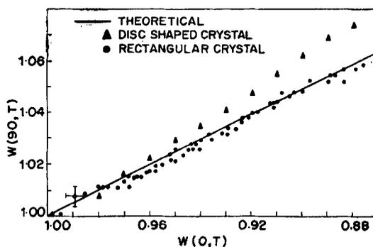
Figure 1. Plot of normalised transverse against longitudinal gamma-ray intensities for two cobalt crystals compared with the theoretical line assuming no closure domains. The range of temperatures covered is 15–80 mK.
