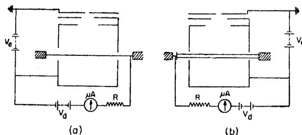
Figure 1. Schematic diagram of the ion sources (a) McClure design and (b) McIlraith design
