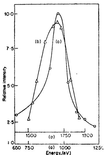
Figure 2. Energy spectra of the ion beams from the two sources (a) McIlraith source and (b) McClure source
