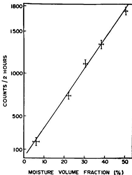
**Figure 2.** Laboratory calibration of the neutron moisture gauge. Medium: alum. Drum size: 15" diam. 15" height
