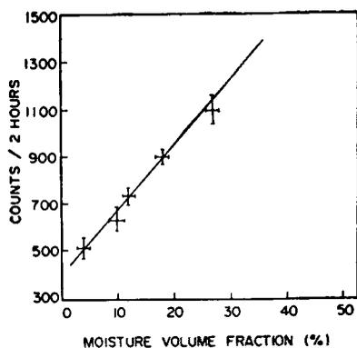
**Figure 3.** Field calibration of the neutron moisture gauge. Soil medium
