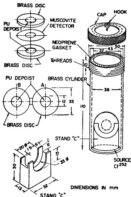
Figure 1. The neutron moisture gauge assembly
