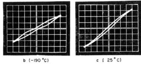
**Figure 2.**  $\chi$ -T curve and hysteresis loops for a 4.6 g sample of SK28. Scale for (b) and (c): one small division on X-axis=50 Oe; on Y-axis=1.0 emu.
