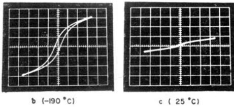
**Figure 1.** Susceptibility *vs* temperature curve and hysteresis loops for a 15.2 g sample of M007. Dashed line in (a) is  $\chi$ -T curve for a normal basalt. Scale for (b) and (c): one small division on X-axis=90 Oe; on Y-axis=0.7 emu.
