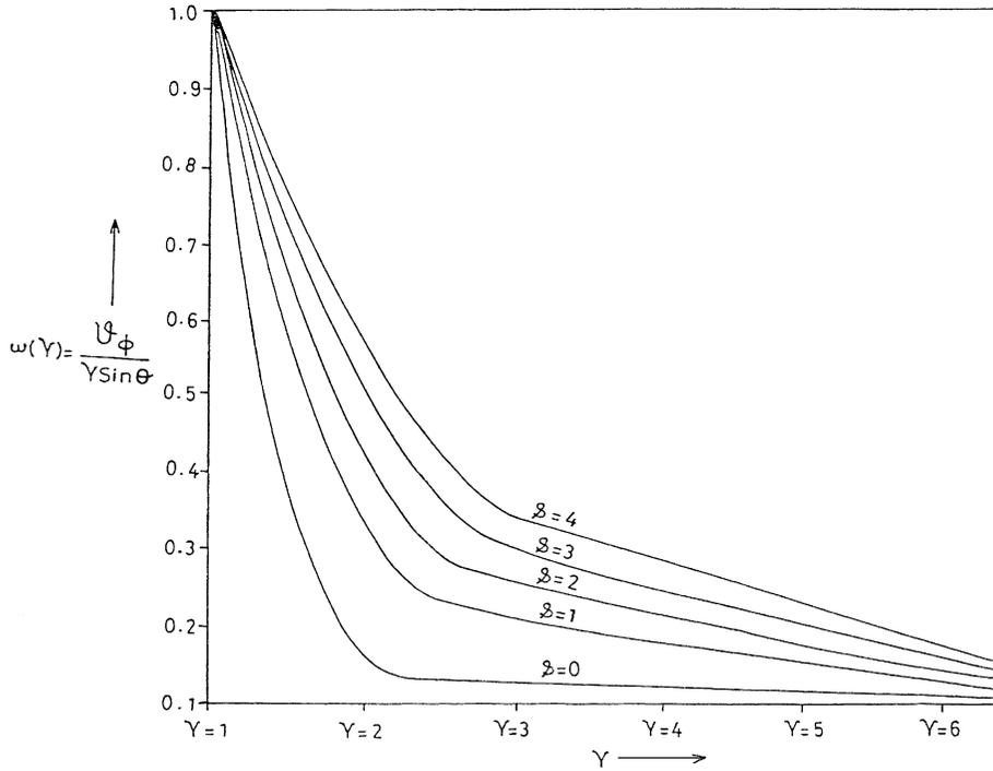
**Figure 1.** Variation of angular velocity  $\omega(r)$  with respect to  $r$  and for various values of parameter  $s$ .
