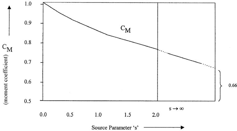
**Figure 2.** Variation of moment coefficient  $C_M$  with respect to source parameter  $s$ .
