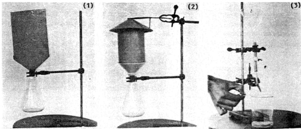
**Figures 1–3.** 1. Bidirectional spore trap used to study the splash-off of the conidia of *R. sorghi* under field conditions. 2. Multidirectional spore trap used to study the splash-off of the conidia of *R. sorghi* under field conditions. 3. Wash-off assembly used to study the wash-off of the conidia of *R. sorghi* by flowing water drops under controlled conditions in the laboratory.
