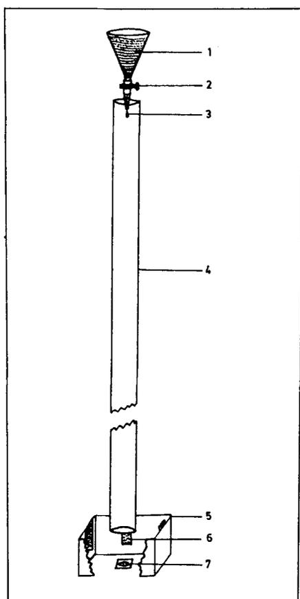
Figure 4. Assembly used for the study of splash-off of the conidia of *R. sorghi* from the infection spots by impacting water drops. (1), Water reservoir; (2), pinch cock; (3), water drop (3 mm diameter); (4), glass tube; (5), splash collecting unit; (6), microscope slide; (7), infected leaf bit mounted on a glass plate.
