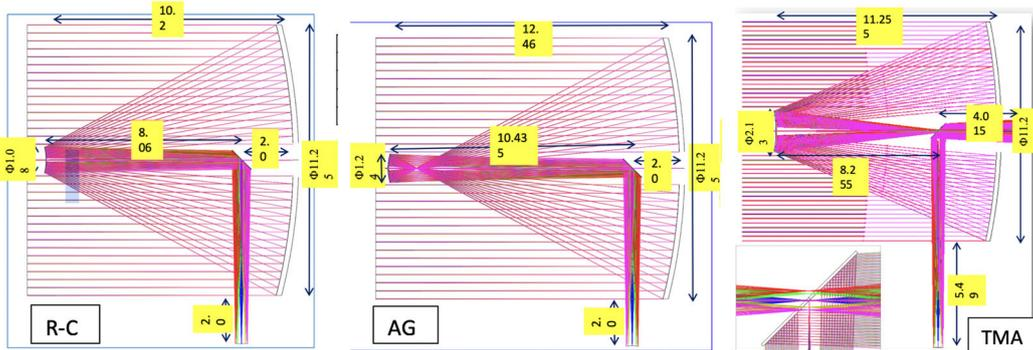
**Figure 1.** Optical layout of the three telescope configurations considered, shown for an  $f/1$  primary as an example. Left: Ritchey–Chretien, middle: aspheric Gregorian and right: three mirror anastigmatic.
