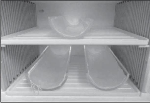
**Figure 6.** Initial experiments using a silicon cloth between the glass sheets and the mandrel to avoid adhesion of molten glass to the mandrel surface. This procedure was later discarded.
