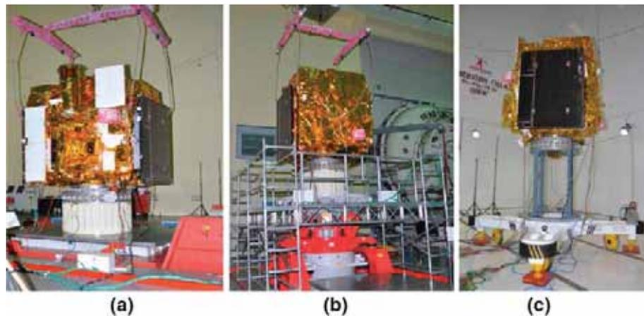
**Figure 34.** Vibration test (a) along lateral axis, (b) along longitudinal axis and (c) acoustic test on AstroSat.
