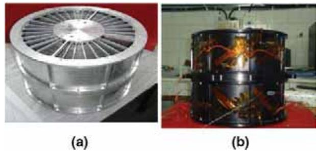
**Figure 20.** (a) Bare optics module of SXT and (b) SXT optics module with thermal elements.
