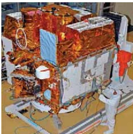
Figure 4. Fully integrated AstroSat spacecraft.
