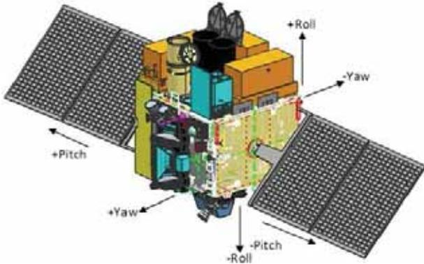
**Figure 1.** AstroSat spacecraft deployed configuration.
