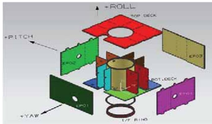
**Figure 11.** Exploded view of the AstroSat structure.
