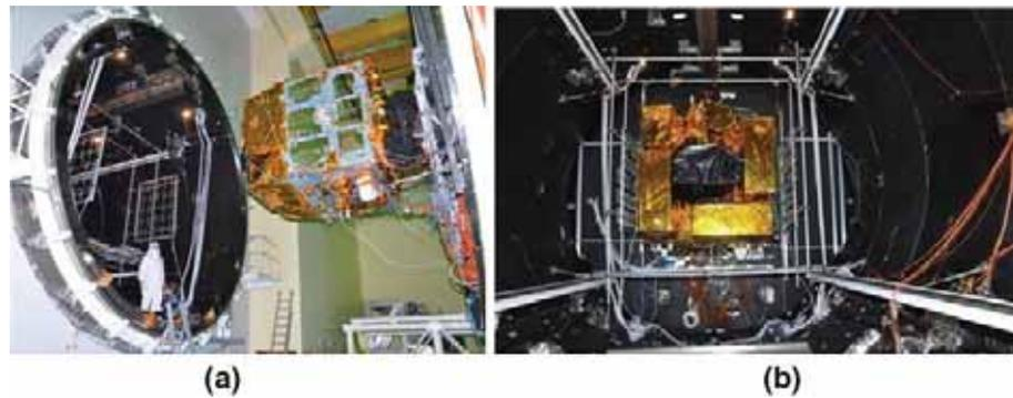
**Figure 33.** (a) Satellite getting loaded inside the TVac chamber, and (b) satellite the inside TVac chamber.
