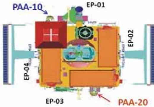
**Figure 28.** AstroSat top view showing accommodation of two-phased array antennae.
