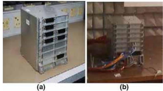
**Figure 27.** Data handling and storage subsystem flight hardware. (a) BDH package and (b) SSR package.
