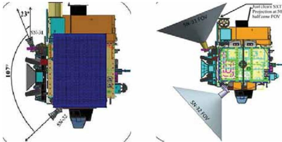
**Figure 10.** Mounting position and FoV of star sensors.
