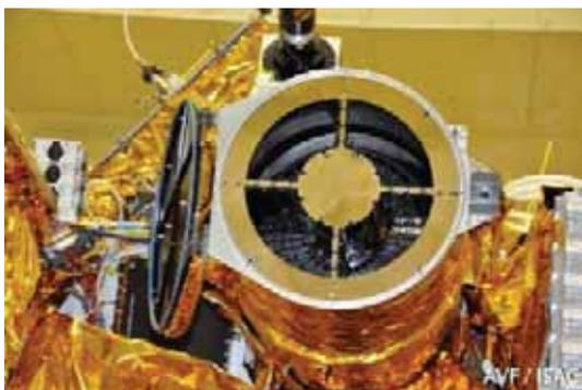
Figure 16. SXT flight model with deployed payload cover.
