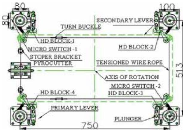
Figure 15. Hold and release mechanism elements.
