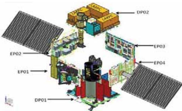
Figure 3. Exploded view of AstroSat configuration.
