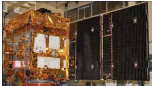
**Figure 13.** Solar array deployment configuration.
