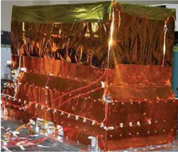
**Figure 18.** Flight LAXPC payload model with thermal control elements.
