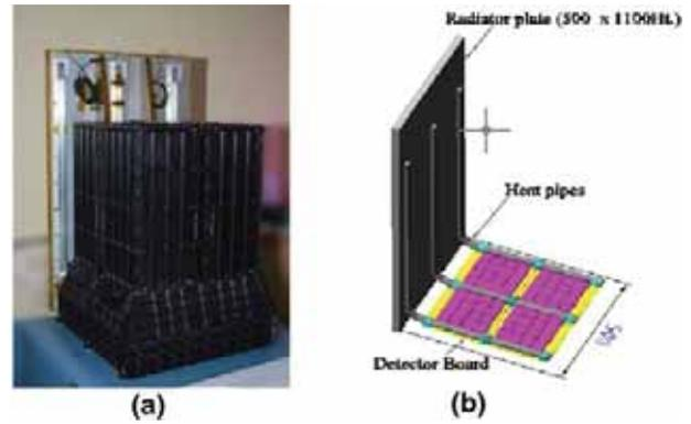
**Figure 19.** (a) CZTI payload assembly, and (b) heat pipe layout (schematic).
