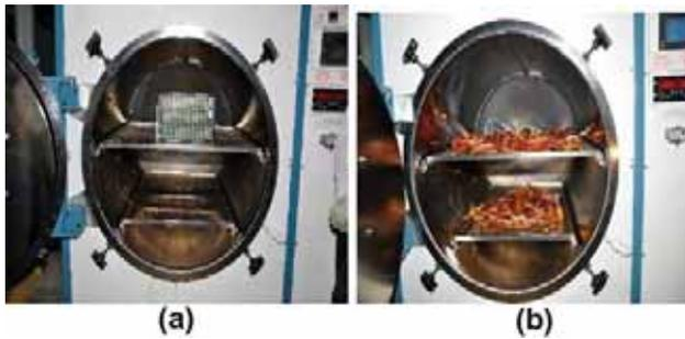
**Figure 32.** (a) Subsystem package baking, (b) harness baking.
