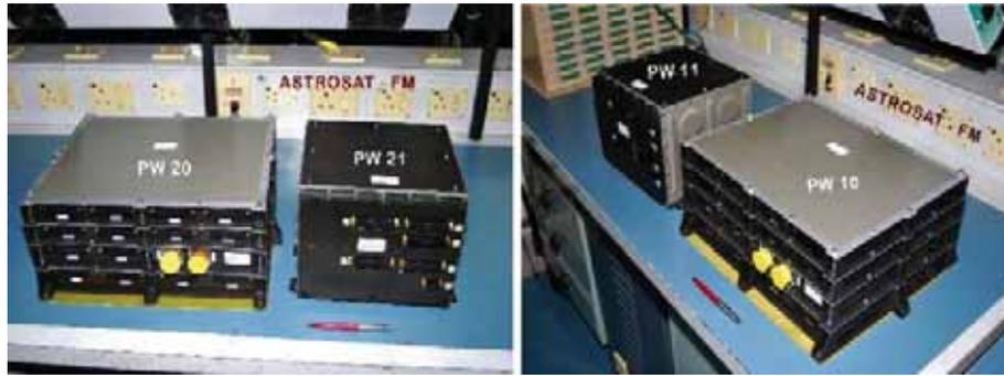
**Figure 24.** Core power packages of power subsystem.
