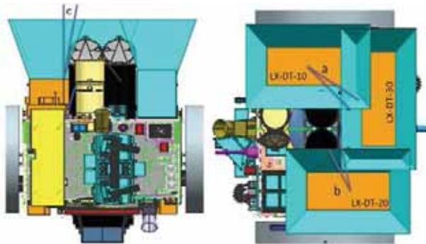
**Figure 7.** FoV of LAXPC payload detectors.
