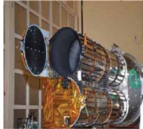
Figure 17. UVIT payload flight hardware with deployed payload covers.
