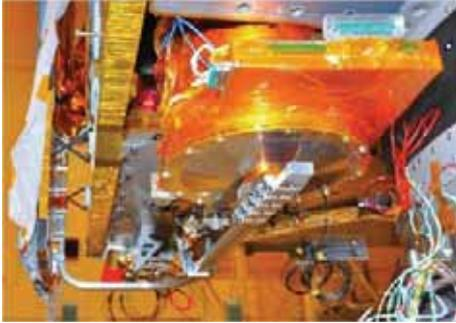
**Figure 21.** Focal plane camera assembly, heat pipe and radiator assembly.
