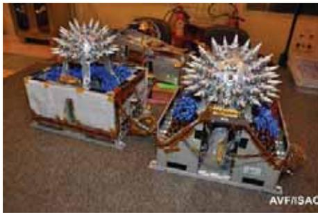
**Figure 29.** Phased array antenna (X-band antenna).
