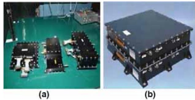
**Figure 31.** (a) X-band and S-band transmitter. (b) SPS package.
