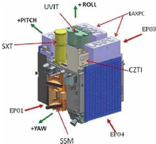
**Figure 2.** AstroSat spacecraft (stowed configuration).
