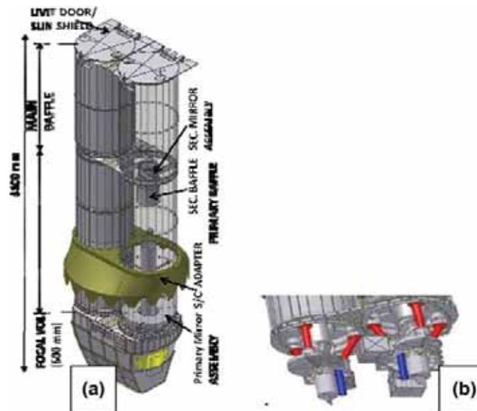
**Figure 22.** (a) UVIT payload assembly with TI mounting adaptor and (b) back focal plane assembly.
