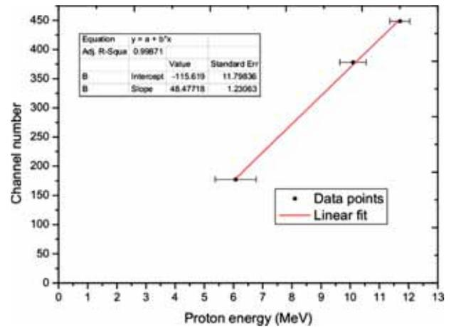
**Figure 3.** Linearity in the peak position for proton beams (linear regression coefficient  $R^2$  of 0.9994).
