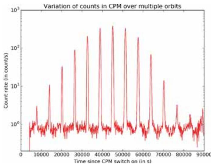
**Figure 4.** Light curve of count as observed by CPM. In the light curve the recurring peaks denote the section of SAA region traversed in an orbit. The highest peak denotes when the satellite ventured deepest into the SAA region. Varying peak height is caused due to the shift of the region of SAA sampled by successive orbits of the satellite.
