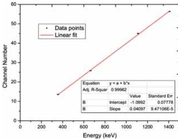
**Figure 2.** Linearity in the peak position for different gamma ray sources (linear regression coefficient  $R^2$  of 0.9955).
