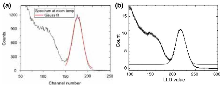
**Figure 1.** Spectrum of radioactive source  $^{137}\text{Cs}$  obtained from CPM. (a) A Multi Channel Analyser (MCA) was used to obtain the spectral information in the Engineering Model (EM). (b) Spectrum for further models was obtained by changing the LLD levels and reading the counts above it. The integral spectrum thus obtained was differentiated to get the spectrum.
