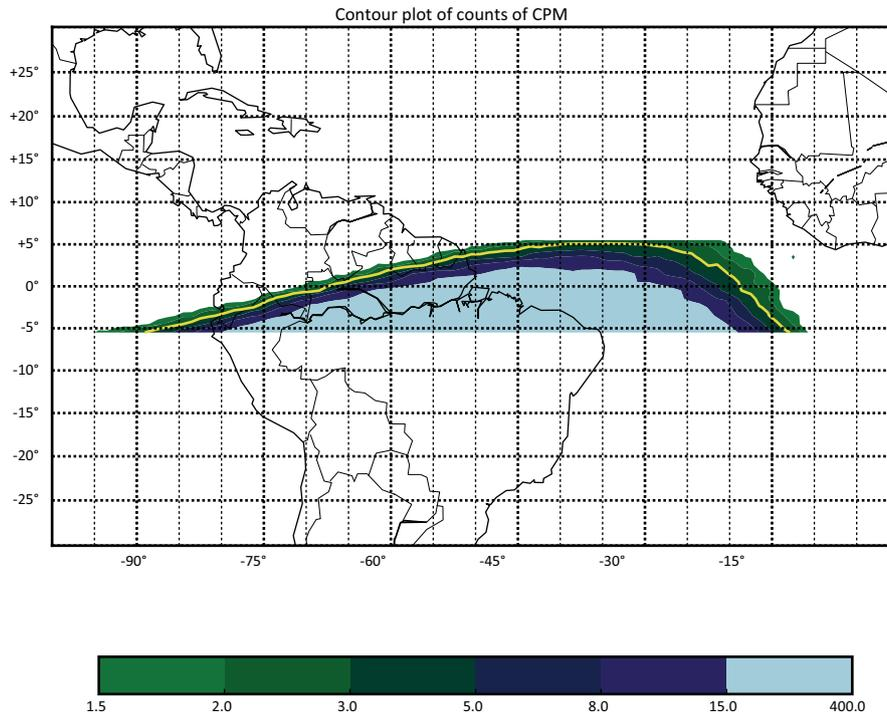
**Figure 5.** Contour maps of SAA region. CPM count rate data for a month was spatially binned and contour maps were generated. The contour maps show variation of count rates from  $\sim 1$  in non-SAA region to 280 counts/s on an average while the peak value reaches 400 counts/s. The boundary for SAA used in Astrosat is 3 counts/s which is shown as a yellow line in the figure. The counts less than 1.5 counts/s have not been shown for clarity of the image.
