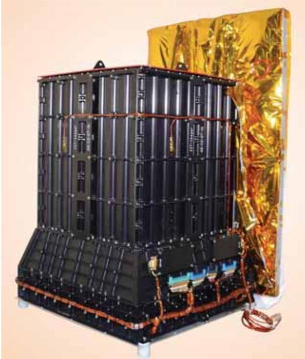
**Figure 1.** The fully assembled cadmium zinc telluride imager before being integrated with the spacecraft.
