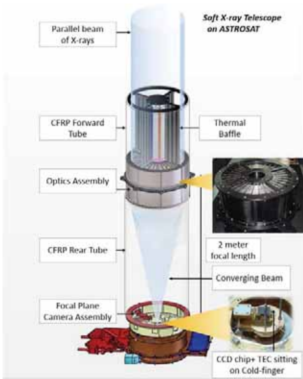
Figure 2. A schematic of the SXT showing the complete assembly of all the components of the SXT.
