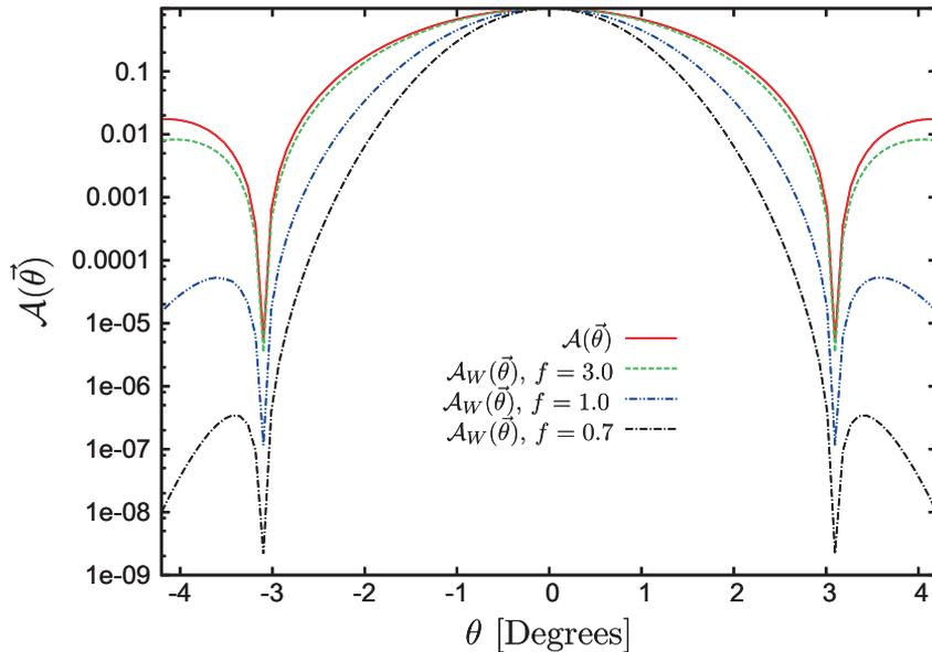
**Figure 1.** The GMRT 150 MHz primary beam  $\mathcal{A}(\theta)$  which has been modelled as the square of a Bessel function. The effective primary beam  $\mathcal{A}_{\mathcal{W}}(\theta)$ , obtained after tapering the sky response for different values of  $f$  is also shown in the figure.
