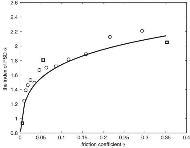
**Figure 4.** The dependence of the spectral index of  $\alpha$  PSD on the friction coefficient  $\gamma$ . The squares denote the values in Table 1 and the solid line represents the best fit of all  $\gamma$  vs.  $\alpha$  points.
