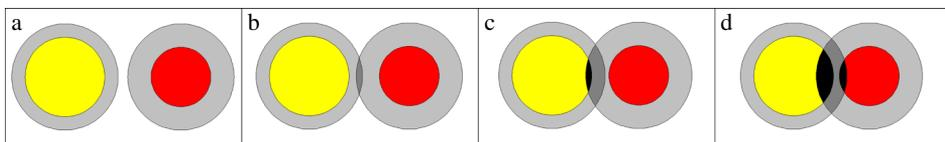
**Figure 1.** Different element–element force situations. The silicate element is yellow with a grey shell. The iron element is red with a grey shell. (a) Elements are not in contact, (b) elements are in contact but neither shell is penetrated, (c) silicate shell has been penetrated, but not the iron shell, (d) both shells have been penetrated.
