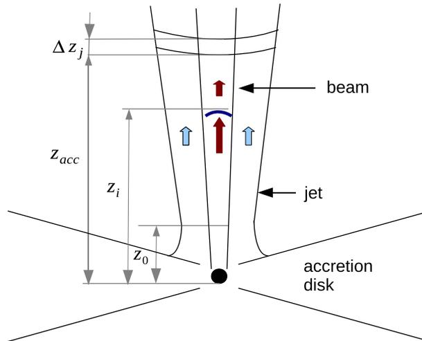
**Figure 1.** Sketch of a two-component jet.  $z_0$  is the beam injection point. Particles are re-accelerated at a distance  $z_{\text{acc}}$  from the black hole, where shocks develop. The thickness of the shocked region is  $\Delta z_j$ .
