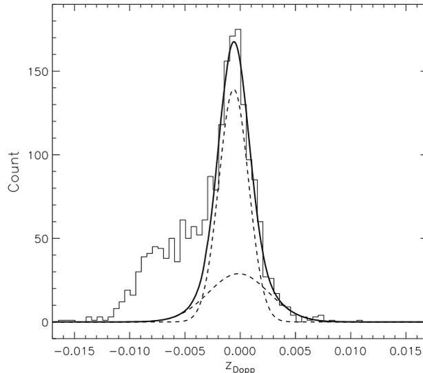
**Figure 3.** A two Gaussian fit to the distribution of Doppler redshifts (calculated with the HW emission redshifts) of the SM12 sample, confined within the range of  $z_{\text{Dopp}} > -0.002$ . The dashed lines represent the two Gaussian components and the thick solid line stands for the fit which is just the sum of the two dashed lines.
