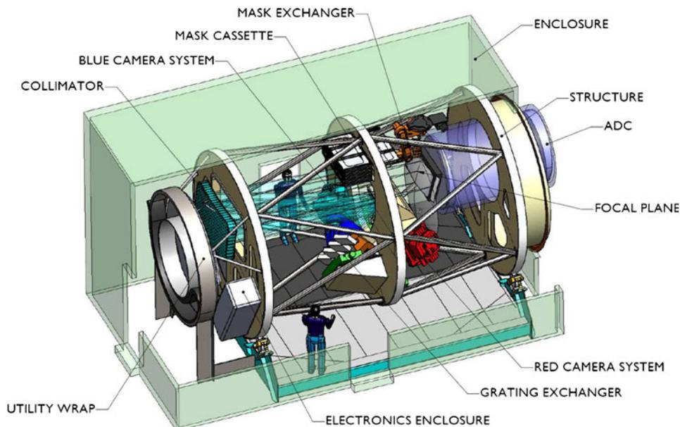
**Figure 5.** Schematic view of MOBIE (Courtesy: Bruce Bigelow, UCO/Lick). The cylindrical instrument assembly is four meters in diameter.
