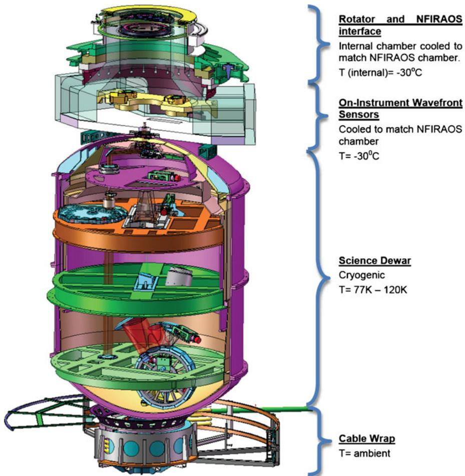
**Figure 4.** Cut-away of the IRIS instrument assembly showing the major instrument sub-assemblies. Only the vacuum-sealed science dewar is maintained at cryogenic temperatures. The remaining modules are cooled to  $-30^{\circ}\text{C}$ , which is the NFIRAOS enclosure temperature. The science dewar contains the IRIS imager and the integral field spectroscopic channels.
