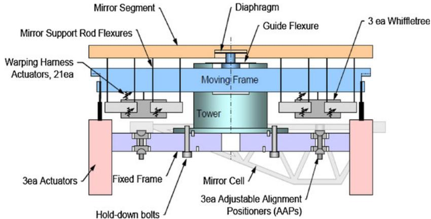
**Figure 4.** Schematic diagram of SSA for TMT.
