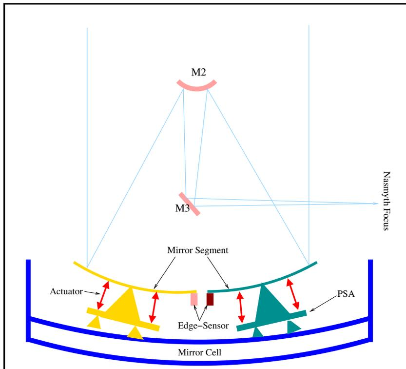
**Figure 1.** Schematic optical layout of TMT. India TMT work packages include about 100 segments of primary mirror and the entire Primary Segment Assembly (PSA): edge sensors, actuators and segments support systems which are shown in the diagram.
