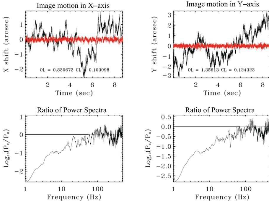
**Figure 4.** A closed-loop tip-tilt correction of the USO-AO system. A closed-loop update rate of 1 kHz is used. Achieved closed-loop bandwidth is about 100 Hz and the improvement in the 'rms' image motion is anywhere between 5 and 25.
