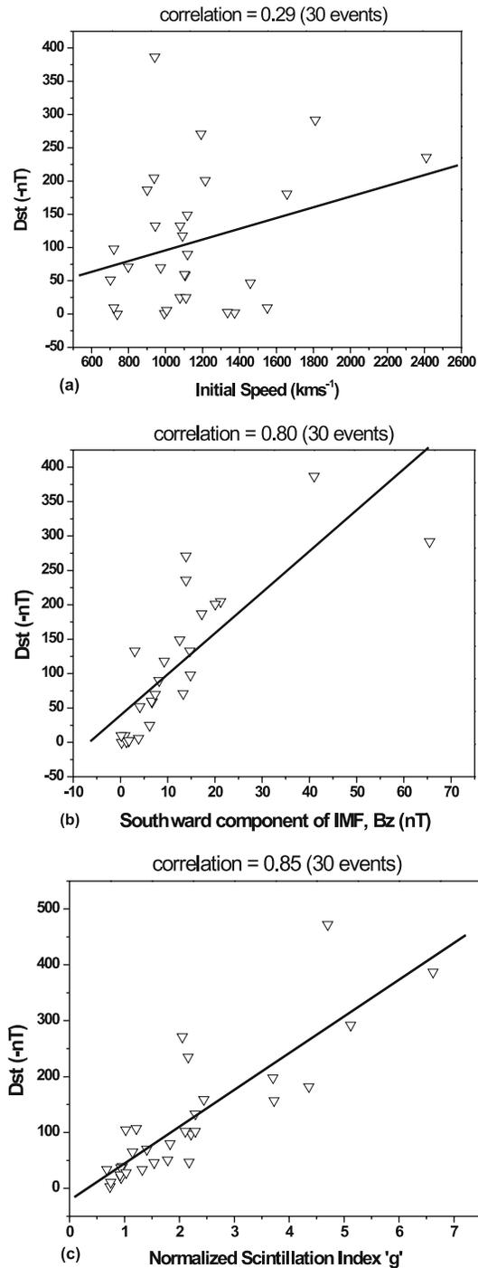
**Figure 3.** Correlation plots of geo-magnetic index Dst and 3 interplanetary parameters, namely: **(a)** initial speed of CME ( $\text{km s}^{-1}$ ) measured by LASCO observations, **(b)** southward component of IMF,  $B_z$  (nT) measured by ACE satellite and **(c)** normalized scintillation index 'g' measured by the IPS observations of radio sources at Ooty.
