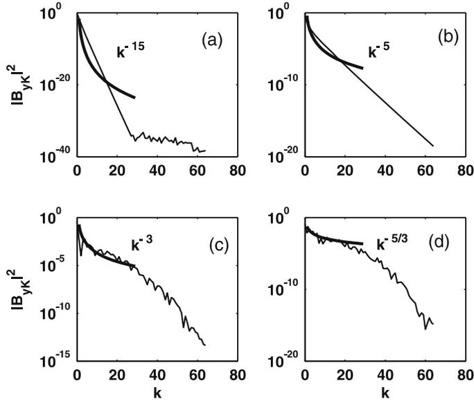
**Figure 2.** Variation of  $|B_{yk}|^2$  against  $k_z$  at  $k_x = 0$  for KAW. (a)  $t = 1.5$ , (b)  $t = 2$ , (c)  $t = 2.5$ , and (d)  $t = 4.5$ . The thick line curve indicates the spectral index scaling.
