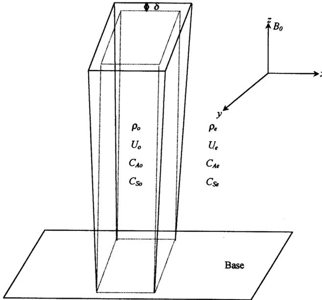
Figure 1. The solar wind flow tube model.
