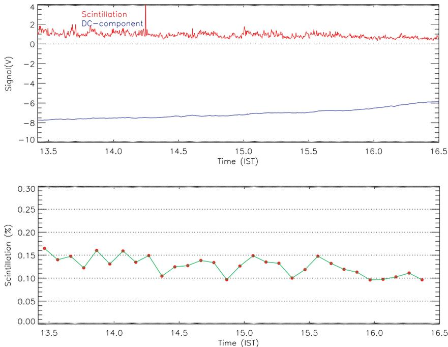
**Figure 3.** Scintillation recorded on March 31, 2005. **Top:** *rms* scintillation integrated over 10 seconds and the average *dc* component. **Bottom:** percentage scintillation averaged over 6 minutes.
