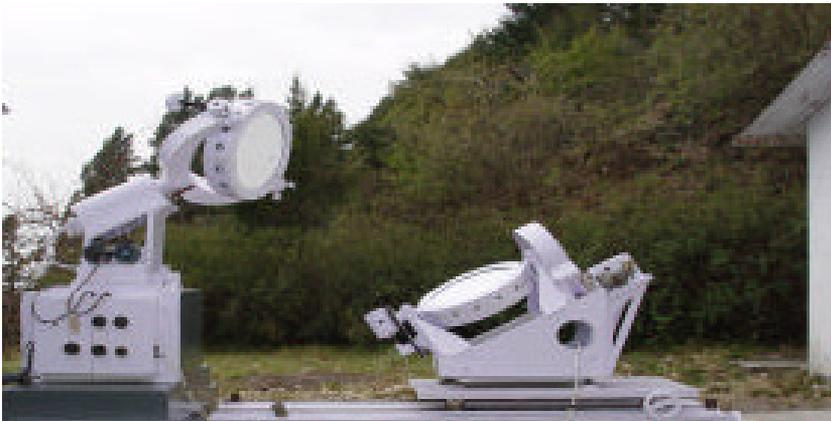
**Figure 1.** The 45-cm coelostat for the 25-cm, f/66 off-axis Skew Cassegrain telescope at ARIES.
