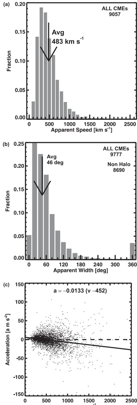
**Figure 1.** CME speed (a), width (b) and acceleration (c) of all CMEs from 1996 to June 2005. The acceleration has a large scatter, but there is a clear trend that the fast CMEs decelerate, while slow CMEs accelerate.
