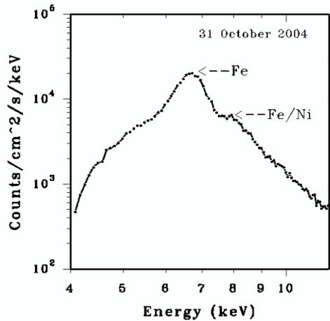
**Figure 2.** Count spectra from Si PIN detector for 31 October 2004 flare at 05:30:59 UT. Note Fe and Fe/Ni line features.
